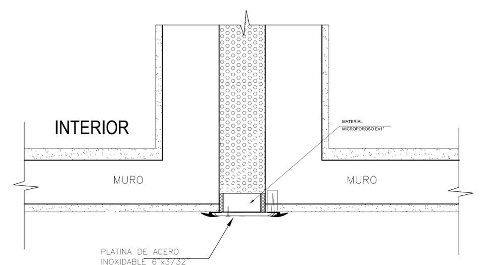
**3 DETALLE TAPAJUNTA EN PARED O COLUMNAS**
